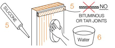
5. Use **only compatible clear silicone** for the sealing
